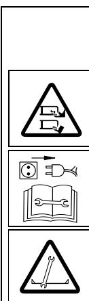
Beware of sharp blades. Blades continue to rotate after the motor is switched off. Before working on the cutters, pull out the mains plug! Keep fingers and feet away from the cutting tools! Before adjusting or cleaning the unit or before checking whether the connection cable is entangled or damaged, switch off the unit and pull out the mains plug. Keep the connection cable away from the tools.
