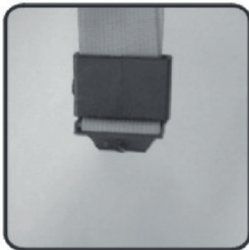
5. Push the plastic clip in the plastic hook hole until in position.
