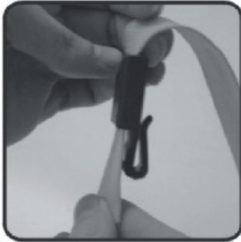
1. Thread the strap down, through the slot of the plastic hook fitting.
